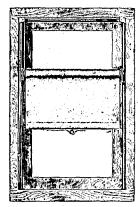
casement, and shut out the best or upper light, and when the top sash was lowered for ventilation it prevented the object de-The sired. Johnson Shade Adjustor, as illustrated herewith, is so adjustable as to obscure any part of the window desired. In the view shown this shade is arranged to protect the middle of the window, thus providing for light above and below, and for ventilation at the same time. These shades
